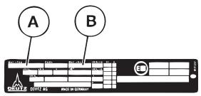
The model type A and the engine serial No. B are given in the engine identification plate.
