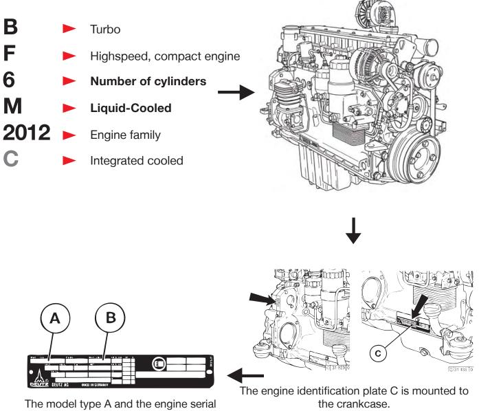
No. B are given in the engine identification plate.
