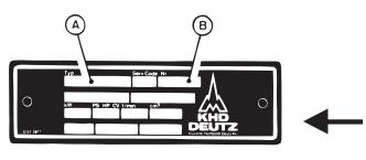
The model type A and the engine serial No. B are given in the engine identification plate.
