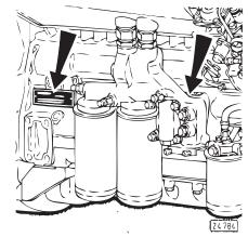
The engine identification plate is mounted to the crankcase at left of the lube filters and in the air cowling. The serial No. is also stamped into the crankcase at the flange for mounting the oil filters.
