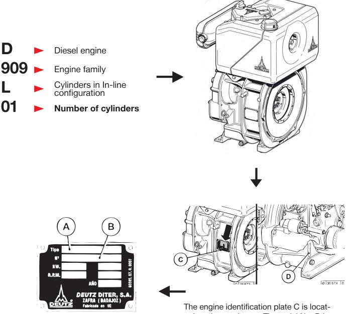
The model type A and the engine serial No. B are given in the engine identification plate. The engine identification plate C is located on the crankcase. The serial No. D is also stamped on the engine block.
