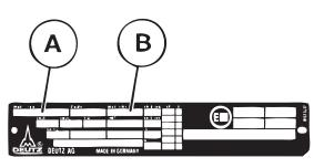
The model type A and the engine serial No. B are given in the engine identification plate. The engine identification plate is mounted to the crankcase. The serial No. is also stamped into the crankcase.
